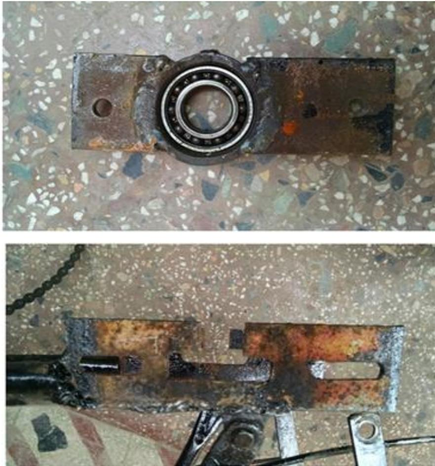
The main function of the bearing is to prevent sliding friction between two parts. Here ball bearing is used with ISO standard 6001. The inner diameter where the bearing casing is fix is 15mm and outer diameter is 30mm. It is also called as pedestal or bearing housing. The second fabricated part in which bearing housing is attached is fixed on both side of rear wheel of the cycle.
