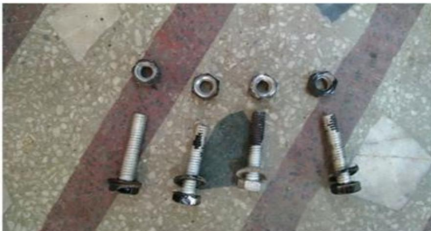
The main function of the bolt is to connect two parts together and give enough strength to the parts. It is four in number. It is used to bolt the bearing housing and the plate for adjustment from both side of the rear wheel gear.
