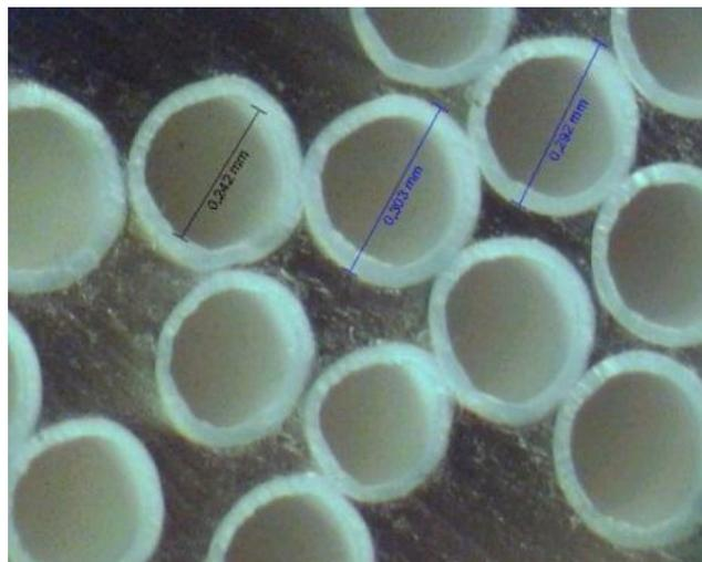
**FIGURE 2: A detailed image of the fibres**
