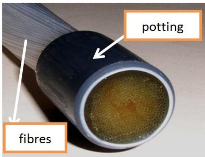
**FIGURE 1: Fibres sealed in the potting**
