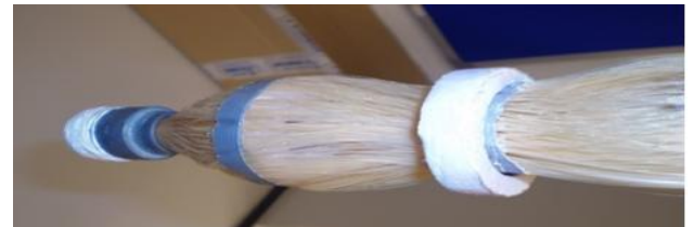
FIGURE 3: A detail of the inner and outer baffles
