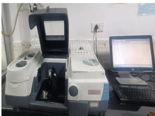
FIGURE 1: FTIR spectrophotometer setup used for functional group identification and structural characterization of FP-1 peptide.
