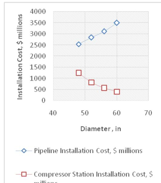
FIGURE V.4 PIPE DIAMETER VS. INSTALLATION COST
