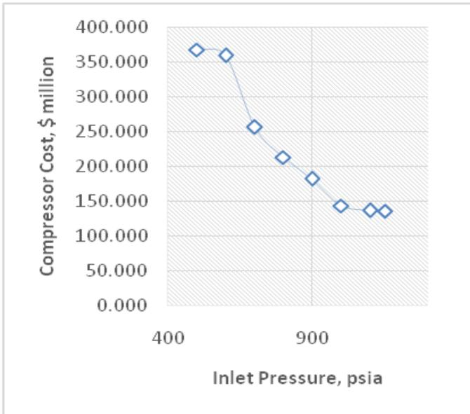
FIGURE V.1 INLET PRESSURE VS COMPRESSOR COST POWER
