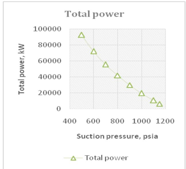
FIGURE V.2 SUCTION PRESSURE VS TOTAL POWER
