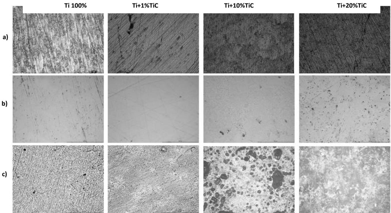
**FIGURE 4: THE SURFACE OF THE THE Ti 100%, (Ti 99%+TiC 1%), (Ti 90% + TiC 10%), (Ti 80% + TiC 20%) SAMPLES AFTER (A) GRINDING, (B) POLISHING, (C) ELECTROPOLISHING; X 100**
