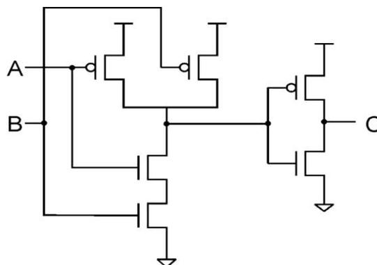
FIG.1 SCHEMATIC DIAGRAM OF CSL AND GATE
