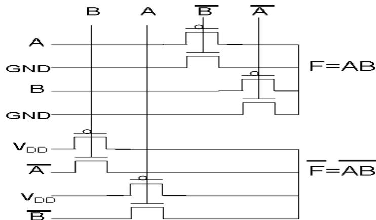
FIG. 5 SCHEMATIC DIAGRAM OF DPL AND GATE
