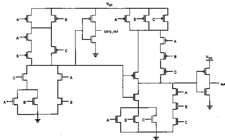
FIG. 2 SCHEMATIC DIAGRAM OF CSL FULL ADDER
