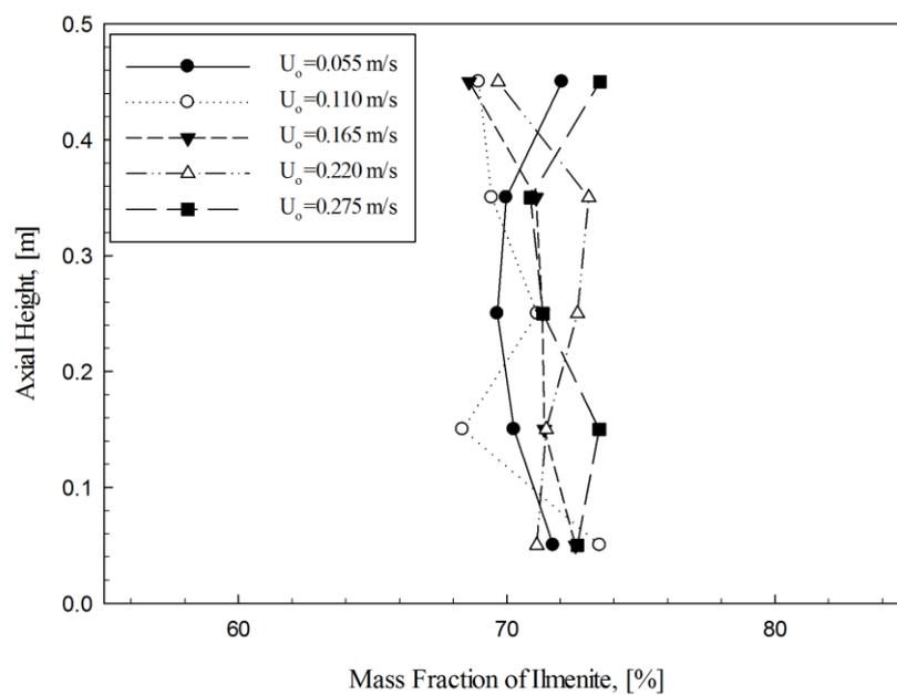
**FIG.3. AXIAL MASS FRACTION OF ILMENITE**
