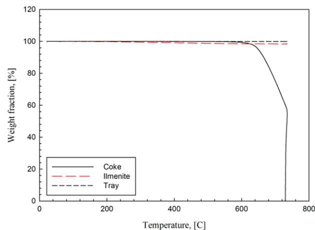
**FIG.3. THERMOGRAVIMETRIC ANALYSIS OF ILMENITE-COKE MIXTURE**
