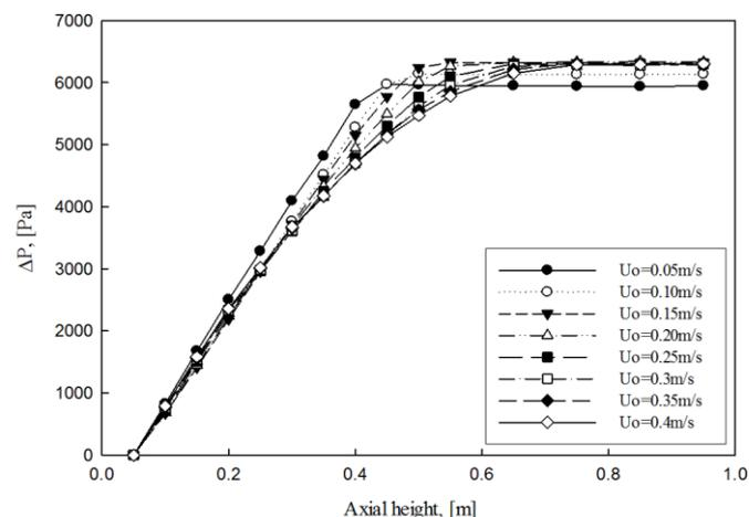
**FIG.4. AXIAL PRESSURE DROPS OF ILMENITE-COKE MIXTURE**
