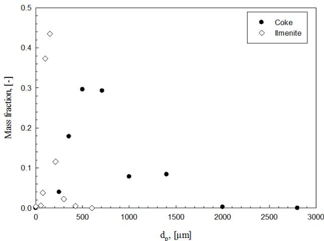
**FIG.2(a). Particle size distribution of ilmenite-coke mixture**
