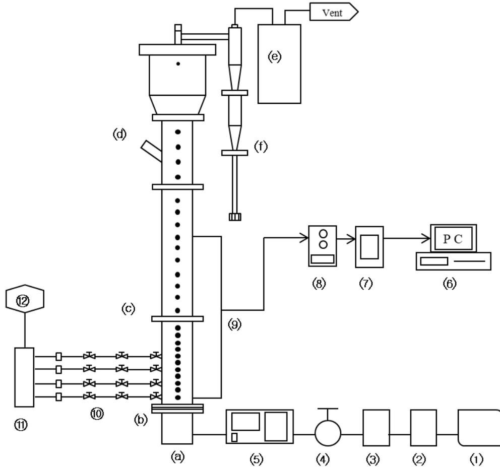
**FIG. 1. Schematic diagram of experimental apparatus: (1) Compressor; (2) Air dryer; (3) Air filter; (4) Regulator; (5) MFC; (6) Computer; (7) A/D converter; (8) Pressure transducer; (9) Pressure line; (10) Sampling line; (11) Vacuum chamber; (12) Vacuum pump; (a) Plenum chamber; (b) Distributor; (c) Main column; (d) Particle inlet; (e) Bag filter; (f) Cyclone.**
