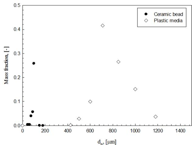
**FIG. 2(b). Particle size distribution of ceramic beads-plastic beads mixture**
