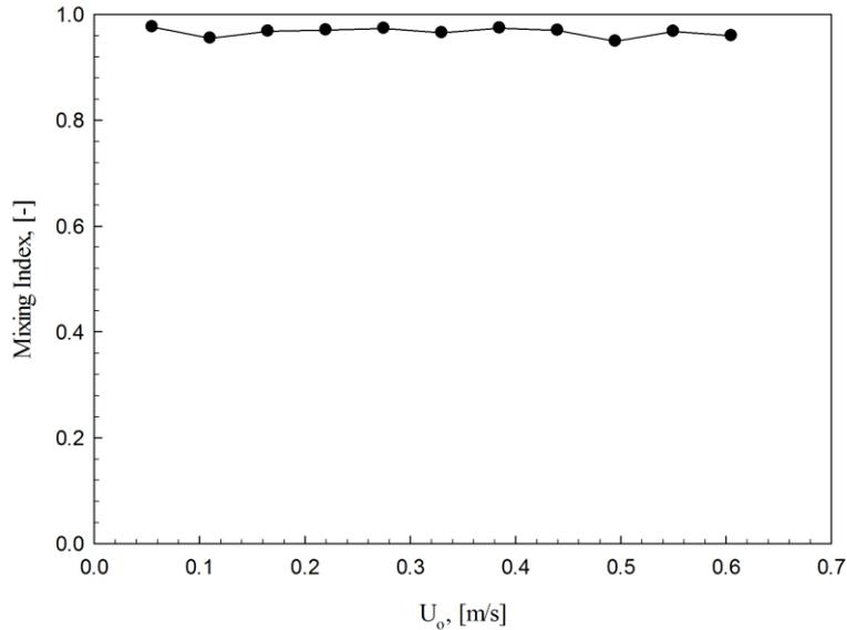
**FIG.7. VARIATION OF MIXING INDEX OF ILMENITE-COKE MIXTURE BED WITH GAS VELOCITY**
