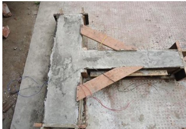
FIG. 3 CASTING OF BEAM COLUMN JOINT
