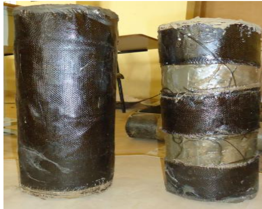
FIG.3 BFRP AND JFRP FULLY AND PARTIALLY WRAPPING.
