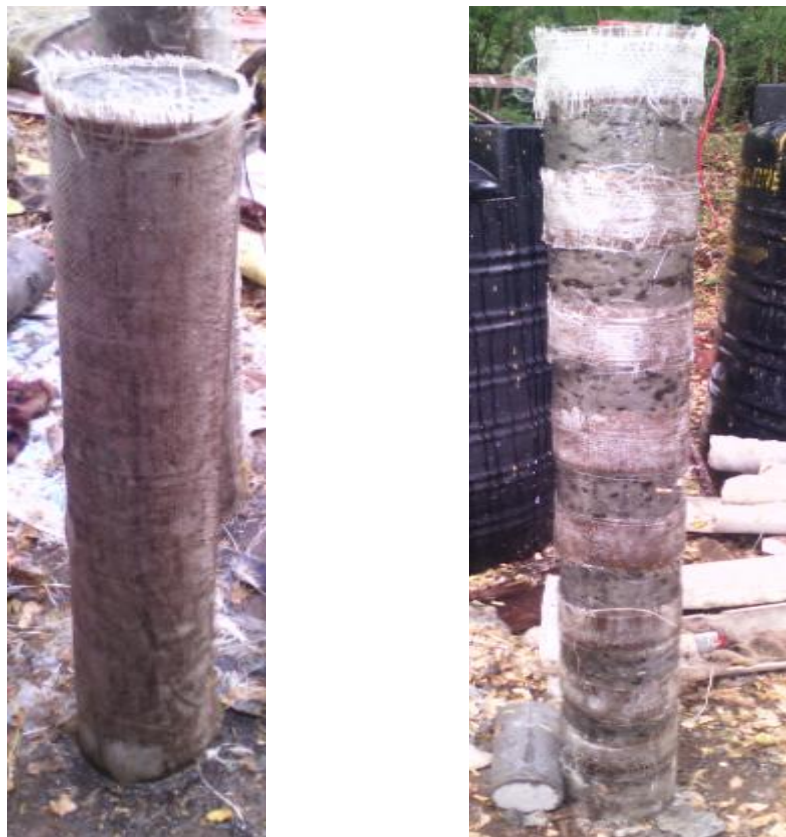
FIG.4: GFRP AND JFRP FULLY AND PARTIALLY WRAPPING
