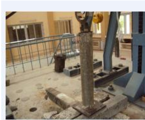
FIG.12.WRAPPING FAILURE OF CIRCULAR COLUMN
