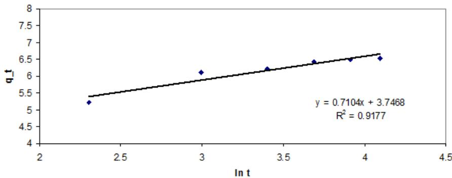
**FIGURE 8: ELOVICH KINETIC MODEL FOR RE-REFINING OF WASTE LUBRICATING OIL USING ACTIVATED UKPOR CLAY**
