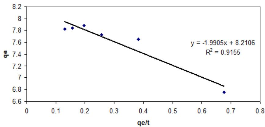
**FIGURE 6: PSEUDO-SECOND ORDER KINETIC MODEL FOR RE-RECYCLING OF WASTE LUBRICATING OIL USING ACTIVATED UKPOR CLAY (EQUATION 5)**
