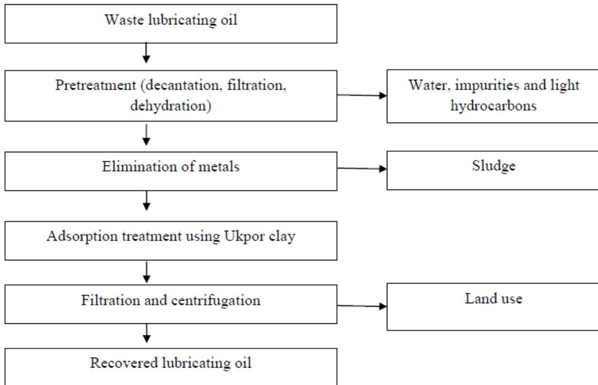
**FIGURE 1: SCHEMATIC DIAGRAM OF WASTE LUBRICATING OIL RE-REFINING PROCESS USING ACTIVATED UKPOR CLAY.**
