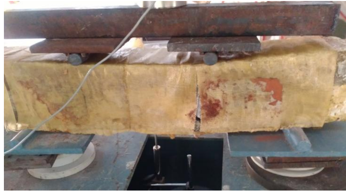
FIG 17 RETROFITTED SPECIMEN AFTER FAILURE
