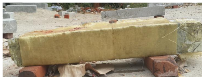
FIG 16 BINDING OF WOVEN MAT OVER THE GFRP SHEETS IN FLEXURAL ZONE
