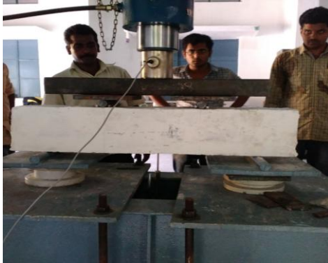
FIG 13 CRACKING OF BEAM BEFORE RETROFITTING
