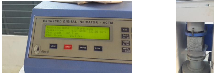
FIG 9 COMPRESSION TEST FOR THE CUBE ON 7 DAYS CURING
