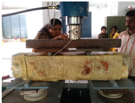
FIG 15 TESTING OF BEAM AFTER RETROFITTING USING GFRP
