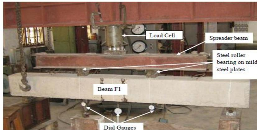
**FIG 8 EXPERIMENTAL SETUP FOR TESTING OF BEAMS**
