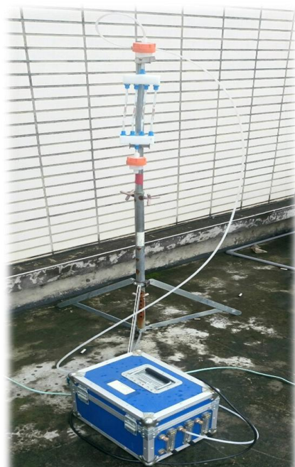
Figure 2-1 four-stage gold amalgamation sampling device
