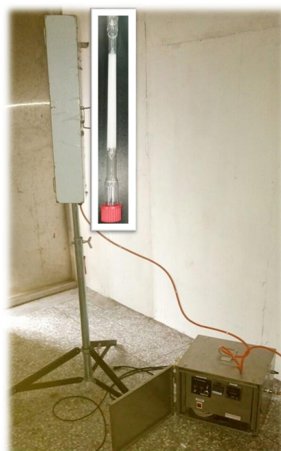
Figure 2-2 denuder sampling device
