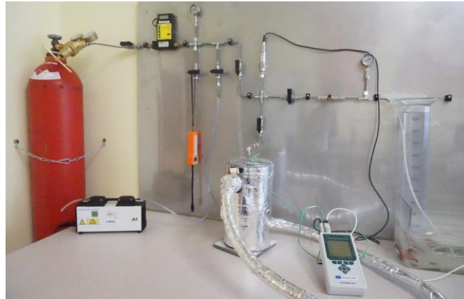
FIG. 6 MEASURING STAND FOR DETERMINING THE STORAGE CAPACITY OF SELECTED METAL HYDRIDE ALLOYS
