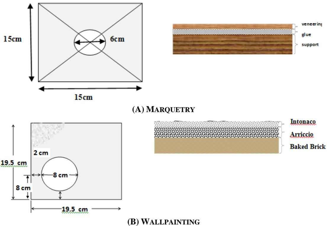
**FIG 4 A) MARQUETRY AND B) WALLPAINTING SAMPLES WITH DEFECT TOPOGRAPHY AND CROSS SECTION SCHEMATICS**
