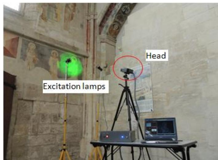
**FIG. 2 CUSTOM DEVELOPED INTERFEROMETRIC SYSTEM FOR ON FIELD APPLICATIONS IN ACTION AT AVIGNON (FR)**
