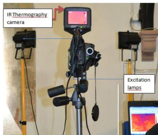
**FIG. 3. ACTIVE INFRARED THERMOGRAPHY SYSTEM FOR ON FIELD APPLICATIONS IN ACTION AT MORVILLE (UK)**
