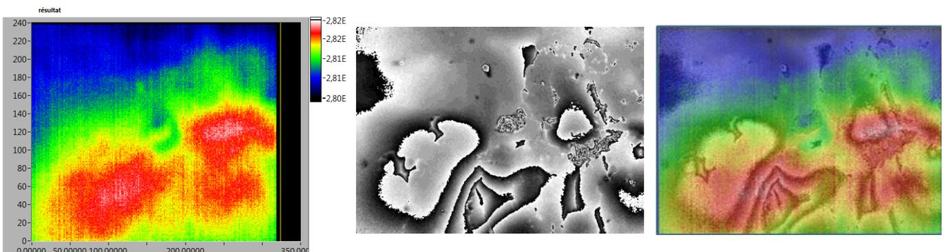
**FIG. 8 EXAMPLE FROM WALL AREA WITH DETERIORATED PLASTER LAYERS, FROM LEFT THE SIRT IMAGE, CENTER THE RAW INTERFEROGRAM AND ON THE RIGHT THE OVERLAPPING.**
