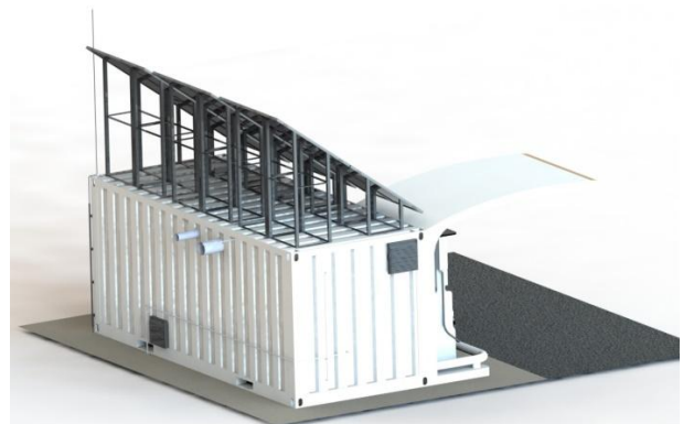
FIG. 8 SINGLE CONTAINER VERSION OF A HYDROGEN FILLING SYSTEM
