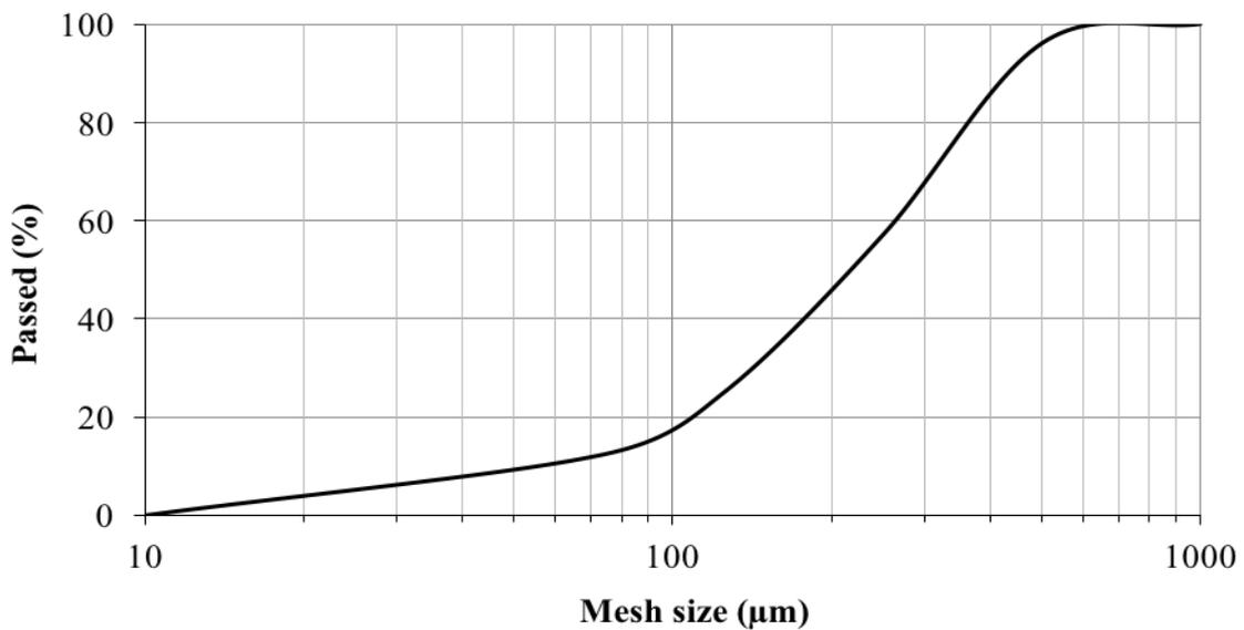
**FIGURE 3. SIEVE ANALYSIS FOR THE BA<sub>2</sub>**
