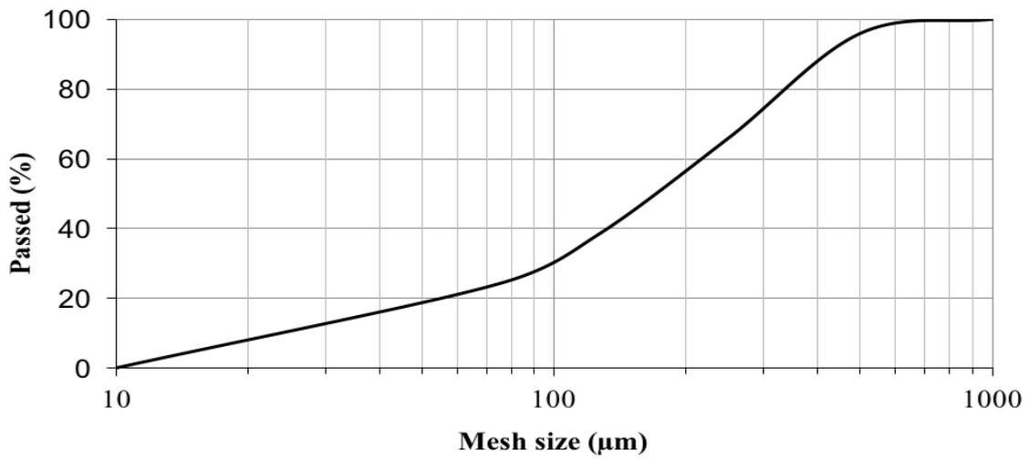
**FIGURE 2. SIEVE ANALYSIS FOR THE BA<sub>1</sub>**
