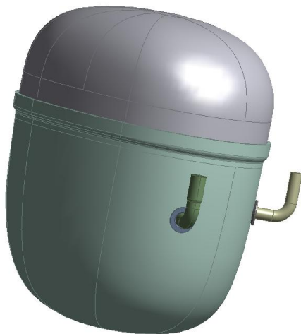
FIG. 5 REDUCED GEOMETRY OF THE COMPLETE COMPRESSOR
