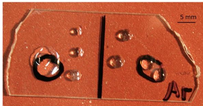
FIG. 6. TYPICAL SHAPE OF WATER DROPS ON UV IRRADIATED PMMA SURFACE. THE IRRADIATED AREA IS ENCIRCLED: LEFT – LABORATORY ATMOSPHERE, RIGHT – ARGON ATMOSPHERE. AVERAGE POWER OF UV IRRADIATION 20 \text{ mW/cm}^2 , IRRADIATION DOSE \sim 4.8 \text{ J/cm}^2 .
