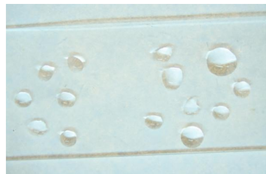
FIG. 8. WATER DROPLETS ON PMMA AFTER TREATMENT IN CHLOROFORM VAPOR. LEFT - UNTREATED AREA, RIGHT - PROCESSED
