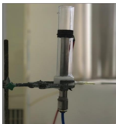
FIG.1. SCHEMATIC STRUCTURE OF PLASMA REACTOR
