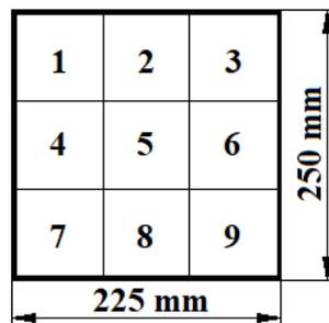
**FIGURE 4: Air duct cross-section with 9 measuring points**
