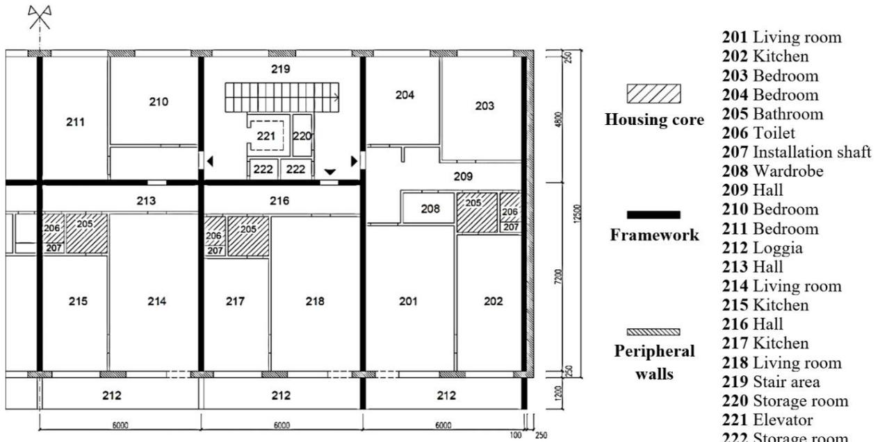
**FIGURE 3: Typical floor of the panel house type T 08B KE [2]**
