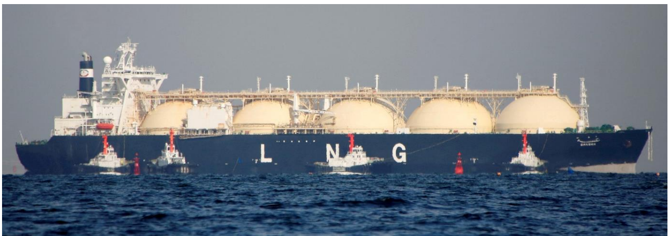
FIGURE 1: Transportation of LNG by tanker [2]
