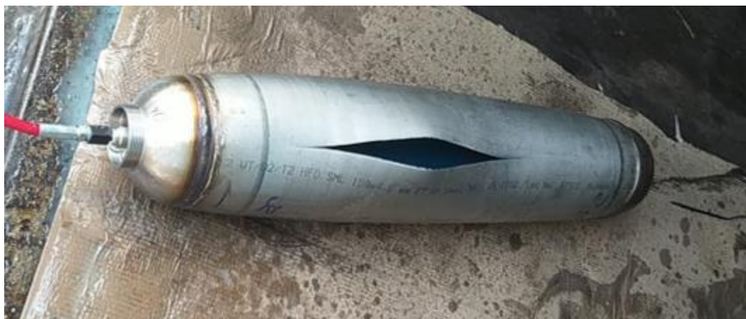
FIGURE 2: Result of hydraulic test until failure
