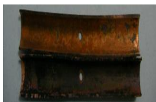
FIGURE2. SURFACE CONDITION 7 DAYS AFTER ELECTROCHEMICAL REACTION OF TAP WATER IMMersed COPPER TU
