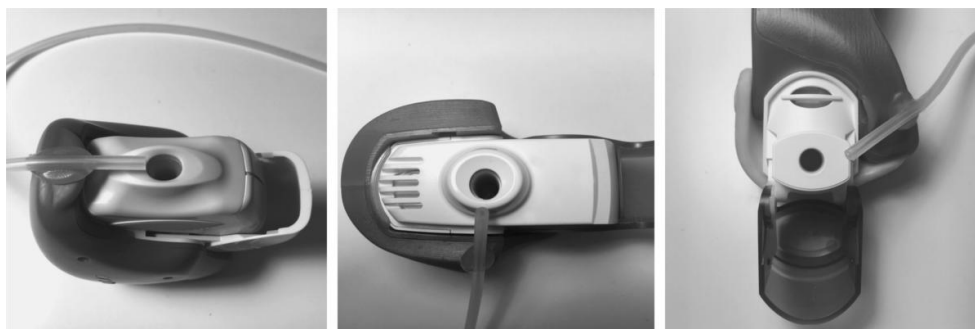
FIG.3 EXPERIMENTAL SETUP WITH DETAIL ON THE SAMPLING TUBE FIXED ON AMIKO®, (LEFT TO RIGHT) FOR ELLIPTA®, NEXTHALER® AND SPIROMAX®.
