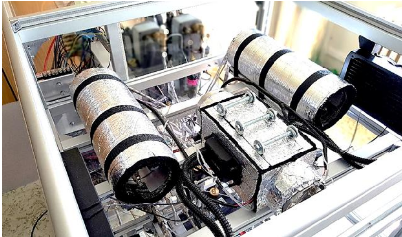
FIGURE 3: View of a tandem pair of MH tanks and an intermediate tank with temperature management
