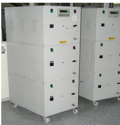
FIGURE 3: Refrigeration compressor testing equipment
