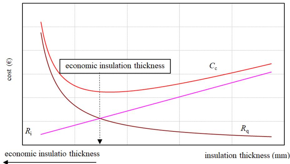
**FIGURE 5: Identification of the economic insulation thickness**
