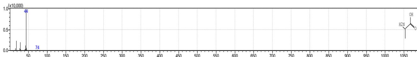
**FIGURE 4: Mass spectrum detected by GC-MS of Alanine.**
