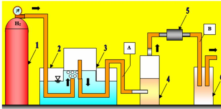
1 – pressure vessel, 2 – outer container, 3 – measuring cylinder, 4 – container with silica gel, 5 – filter, 6 – drain container SiO<sub>2</sub>
