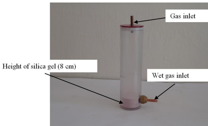
**FIGURE 6: Vessel with silica gel**
