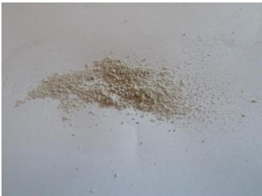
**FIGURE 3: Ground sample of silica gel**
