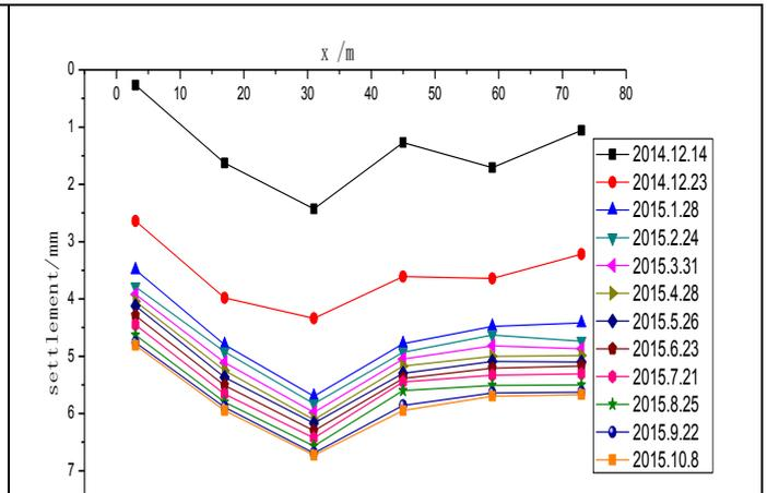
**FIG. 3 SETTLEMENT CURVE OF THE SOUTH SIDE OF FOUNDATION PIT**
