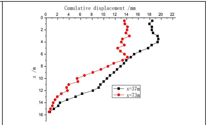
**FIG. 7 CUMULATIVE HORIZONTAL DISPLACEMENT CURVE OF THE SOUTH SIDE OF FOUNDATION PIT**
