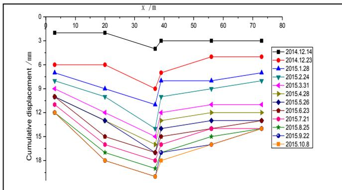
**FIG. 4 HORIZONTAL DISPLACEMENT CURVE OF THE NORTH SIDE OF FOUNDATION PIT**
