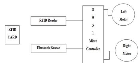
FIG.6. BLOCK DIAGRAM OF ROBOT NAVIGATION
