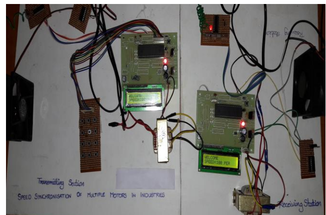
FIG8. SPEED SYNCHRONIZATION OF MAIN AND RECEIVING MOTOR
