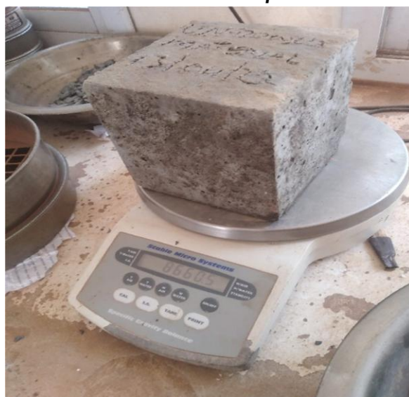
FIGURE 6: Cube being weighed
