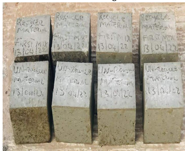
FIGURE 4: Casted cubes after 24 hours
