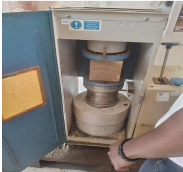
FIGURE 7: Crushing of cube in the Compressive Testing Machine
