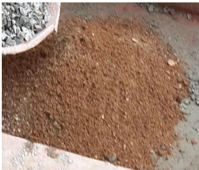
PLATE 11: Photograph showing river sharp sand used as fine aggregate in the concrete mixtures
