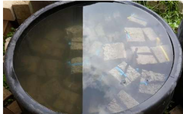
Plate 17: Photograph showing freshly cast concrete cube specimens in moulds during the curing process
