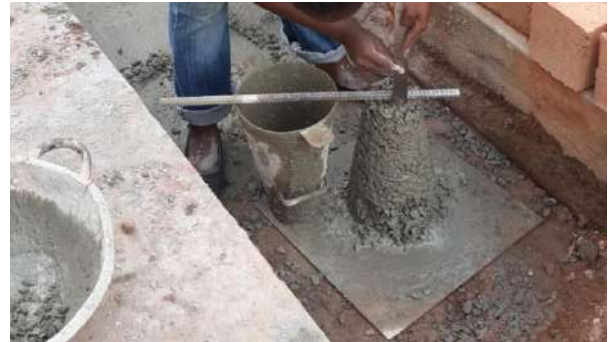
Plate 16: Photograph showing a slump test being performed to evaluate the workability of fresh concrete
