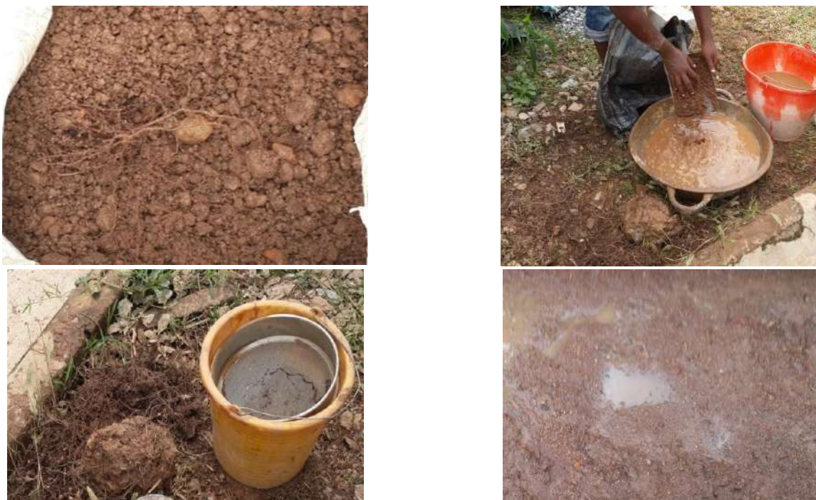
Plate 8: Photograph showing unwashed natural gravel together with debris, roots, and silt removed during the cleaning process
