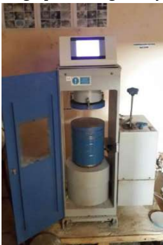
Plate 18: Photograph showing concrete cube specimens being tested in a compression testing machine to determine compressive strength
