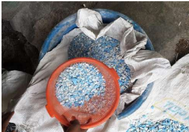
PLATE 3: Photograph showing finely crushed WPET particles obtained after sieving through a 6.70 mm mesh sieve
