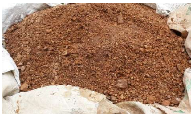
Plate 9: Photograph showing washed gravel used as coarse aggregate in concrete production
