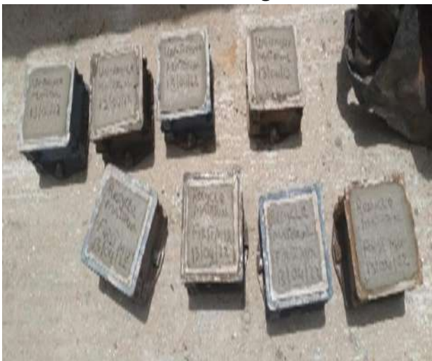
FIGURE 3: NAC and RAC casted in moulds
