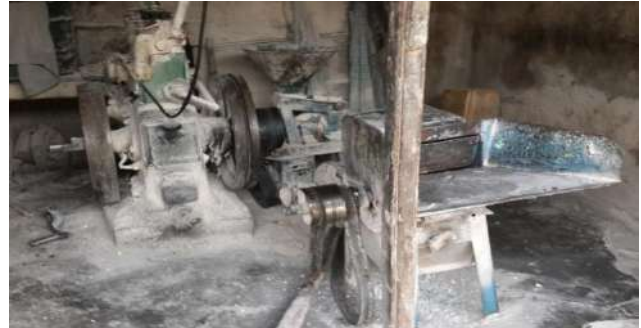
PLATE 2: Photograph of the hammer mill machine used to crush waste polyethylene terephthalate into smaller particles suitable for concrete production
