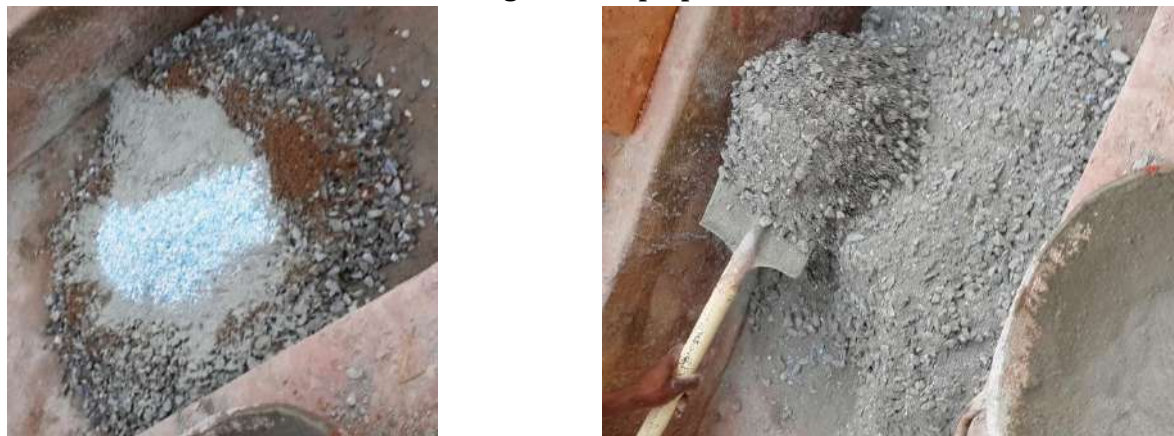
Plate 15: Photograph showing a freshly mixed concrete batch containing 8% WPET replacement
