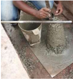
Plate 16: Photograph showing a slump test being performed to evaluate the workability of fresh concrete
