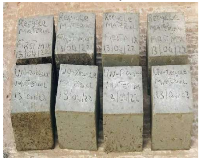
FIGURE 4: Casted cubes after 24 hours
