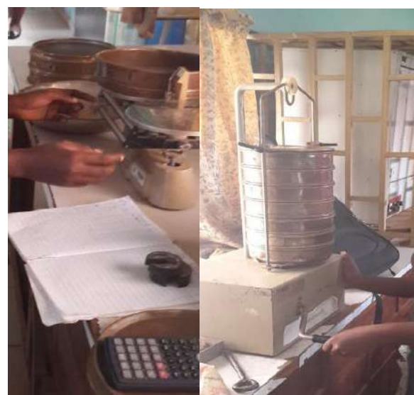
PLATE 5: Photograph showing the sieve analysis equipment, including sieves, weighing balance, and WPET sample used for particle size distribution testing
