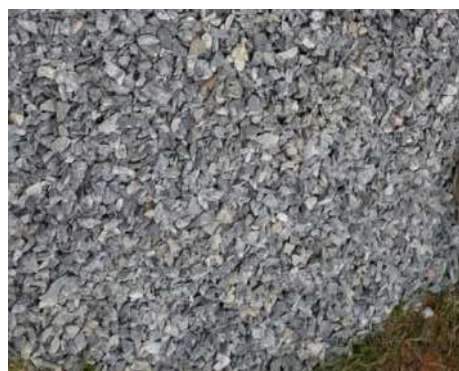
Plate 10: Photograph showing granite aggregate used as coarse aggregate in concrete production
