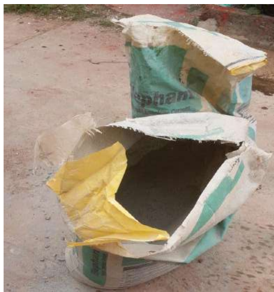
PLATE 12: Photograph showing Ordinary Portland Cement (Grade 32.5N) used for concrete production
