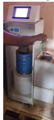
Plate 18: Photograph showing concrete cube specimens being tested in a compression testing machine to determine compressive strength
