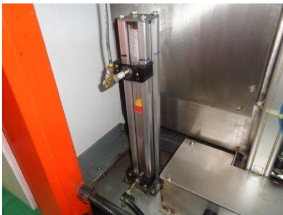
FIG. 11: LEVEL SENSOR IN THE MACHINE
