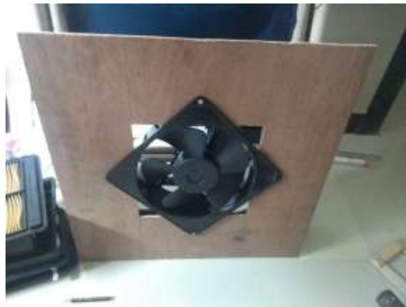
Fig 7. Suction Fan mounted on Plywood
