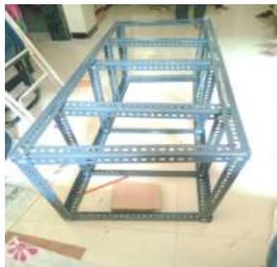
Fig 5. Slotted Angles Structure
