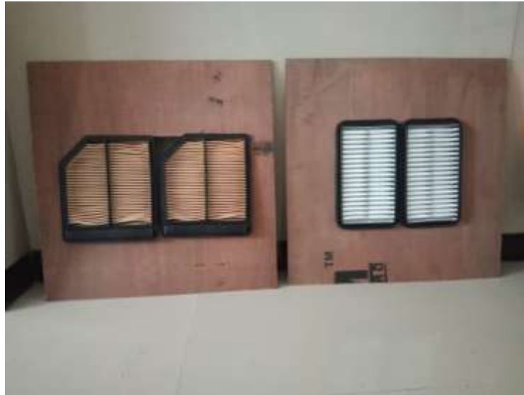
Fig 6. Filters mounted on Plywood Sheet
