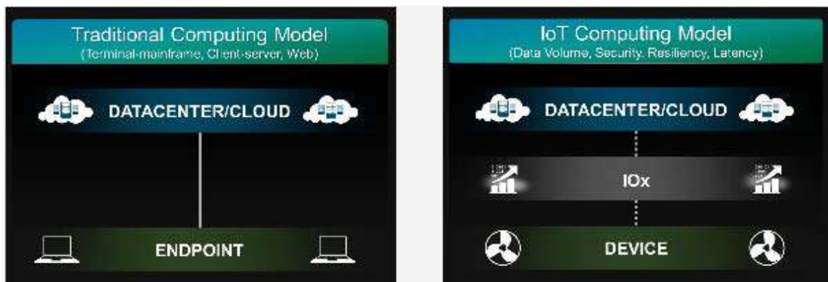
Fig. 3. Cloud and Fog Architecture
