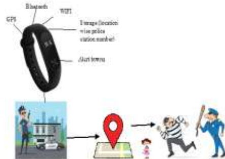
Fig 3: Working of smart band
