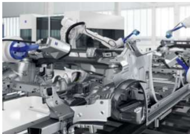
Figure 11: Optical measurement of automotive body dimensions using laser triangulation sensors to achieve detection and isolation of faults.
