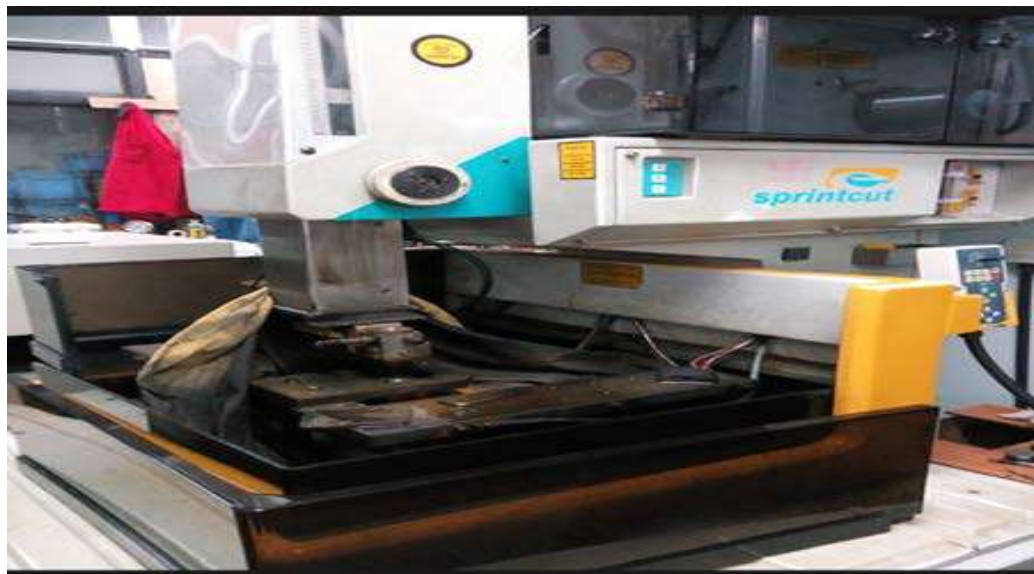
Fig.3.3: Working zone of Wire electrical discharge machining
