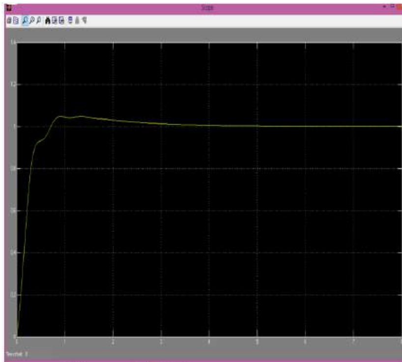
Fig.8 Simulink output of bus suspension system using PID controller
