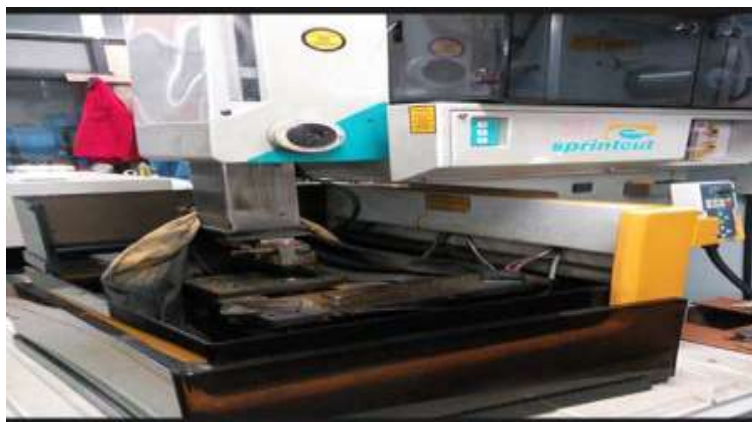
Fig.4: Working zone of Wire electrical discharge machining
