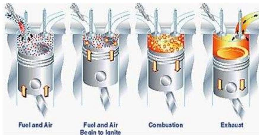
Fig. 2 Homogeneous charge compression ignition combustion principle
