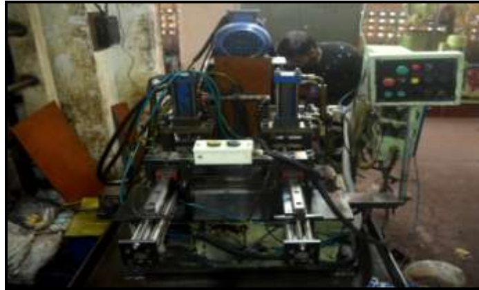
Fig.3.2 Two spindle drilling Machine (BDR-01)
