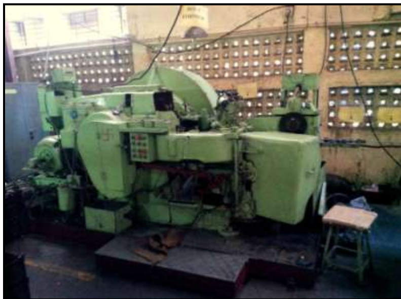
Fig.3.1: 3/8 National Bolt Former Machine
