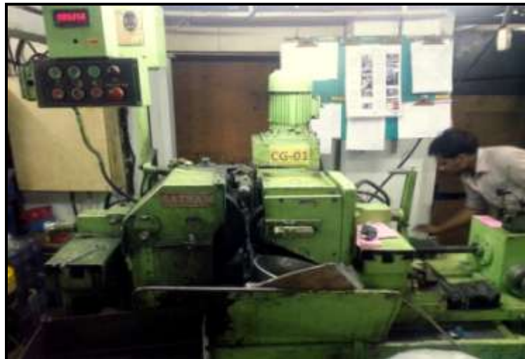
Fig.3.4 Centerless Grinding Machine (CG-01)
