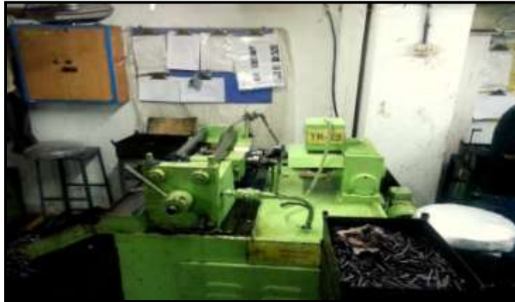
Fig.3.3 Thread Rolling Machine (TR-13)
