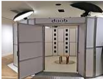
FIGURE 2:3D models can be generated from 2D pictures taken at a 3D photo booth.
