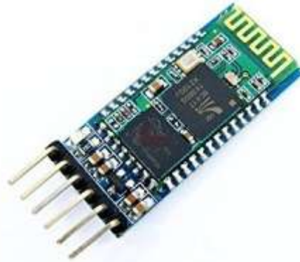
FIGURE 3:- Bluetooth module HC-05
