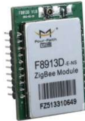
FIGURE 5 -F8913 Embedded ZigBee Module
