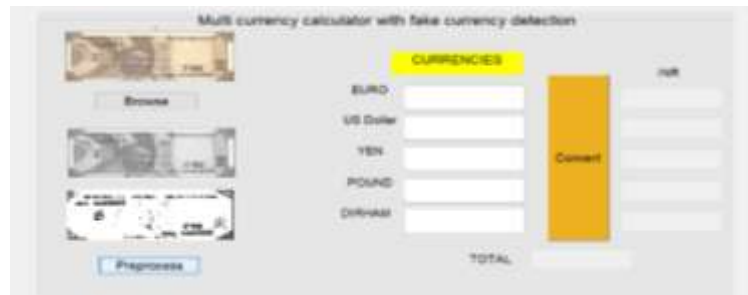
FIGURE 3: GUI for Pre-processing of 10/- Rupee Note with the Calculation of Overseas Currencies into INR
