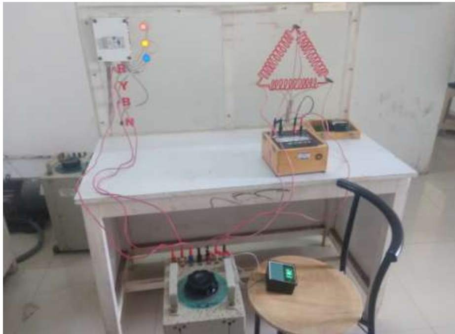
FIGURE 2: Retardation test set up in laboratory for Experiment
